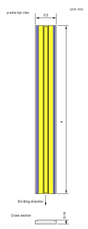
Since the laser bare chip has no marker indicating the light emitting direction, it is displayed on the packing case. At mass production, markers are displayed on laser bare chip.
